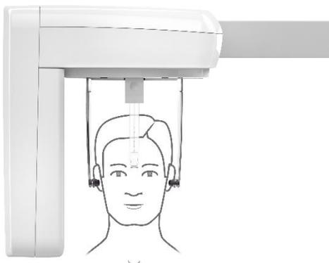
Grasp the ear plug holders at the top and simultaneously slide them together. The ear plugs are positioned on the patient's outer auditory passage.
