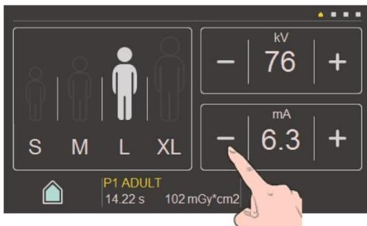
If the preset kV/mA combinations do not provide a satisfactory result, it is possible to set the kV/mA values manually in all programs. Increase or decrease kV and mA values by touching icons “+” or “-”.
