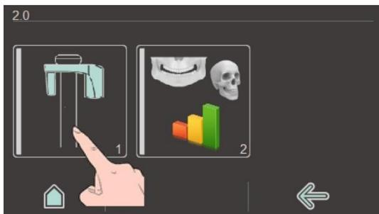
By pressing the icon on the left it is possible to access the menu containing the information of the specific unit (S/N, FW release, touch-screen FW release, etc.).
