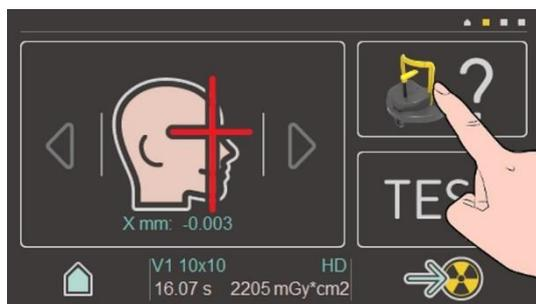
Press and keep pressed the button "positioning tool" in the upper right part of the touchscreen.
