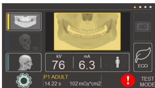
If an error message is present, the icon “Error” is shown in the bottom-right part of the control panel, as illustrated in the side image.
