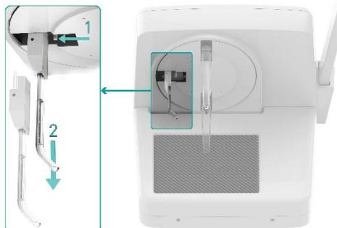
Remove the nasion support by acting on the release pin as illustrated in the side image.
