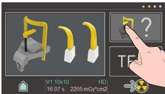
Check that the positioning tool inserted in the device is one of those needed for the selected exams, shown in the main window of the touchscreen.
