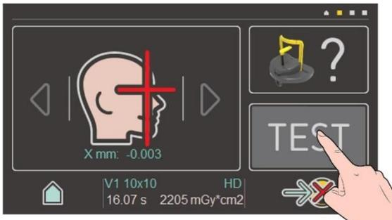
The test cycle is executed without radiation. The test cycle is used to check that the unit is functioning correctly and to ensure that a complete, uninterrupted cycle is possible.
