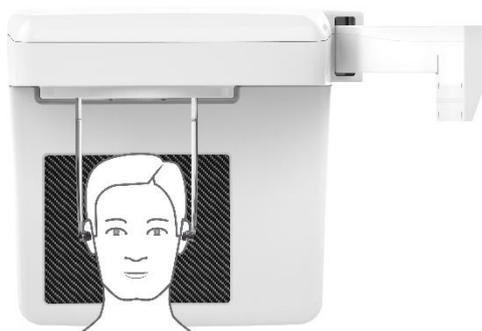
Grasp the ear plug holders at the top and simultaneously slide them together. The ear plugs are positioned on the patient's outer auditory passage.
