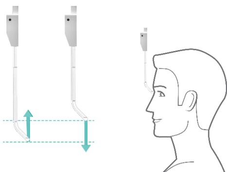
Grasp the plastic part of the nasion support and adjust the nasion support height by bringing it up/down.
