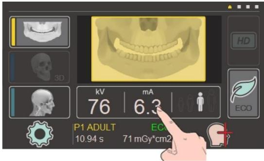
It is possible to select patient size or adjust manually the technical parameters kV and mA (mAs only for cephalometric programs) by pressing the “kV/mA/size” button, in the middle of the display home page.
