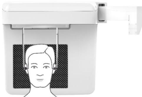
The configuration of the craniostat for Antero-Posterior program is indicated in the side image. Turn the ear plug holder, in order to have ear plug as illustrated in side image. Grasp the holders at the very top with both hands. Push the holders simultaneously outwards as far as they will go. Insert the protective caps for ear plug.
