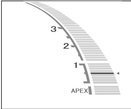
5. Check that all the canal length indicator bars on the display are lit, the word "APEX" flashes and audible beep becomes continuous.
