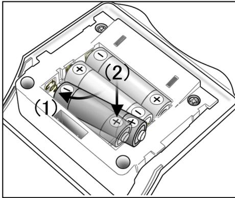
3. Take out the old batteries and replace them with new ones. Make sure the plus and minus poles are correctly lined up.
