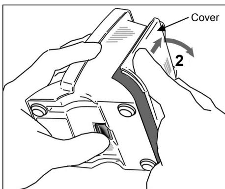
1. Hold the cover and slide the stopper on the bottom towards the liquid crystal display.
