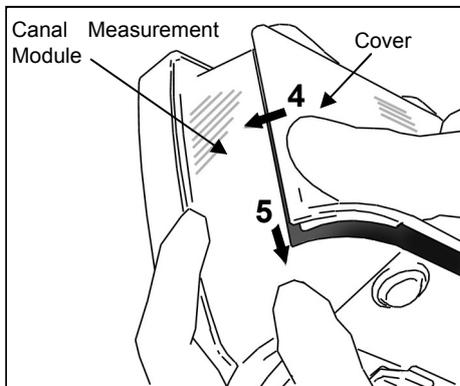
4. Line up the tabs on the cover with the notches on Canal Measurement Module and slide the cover on.
