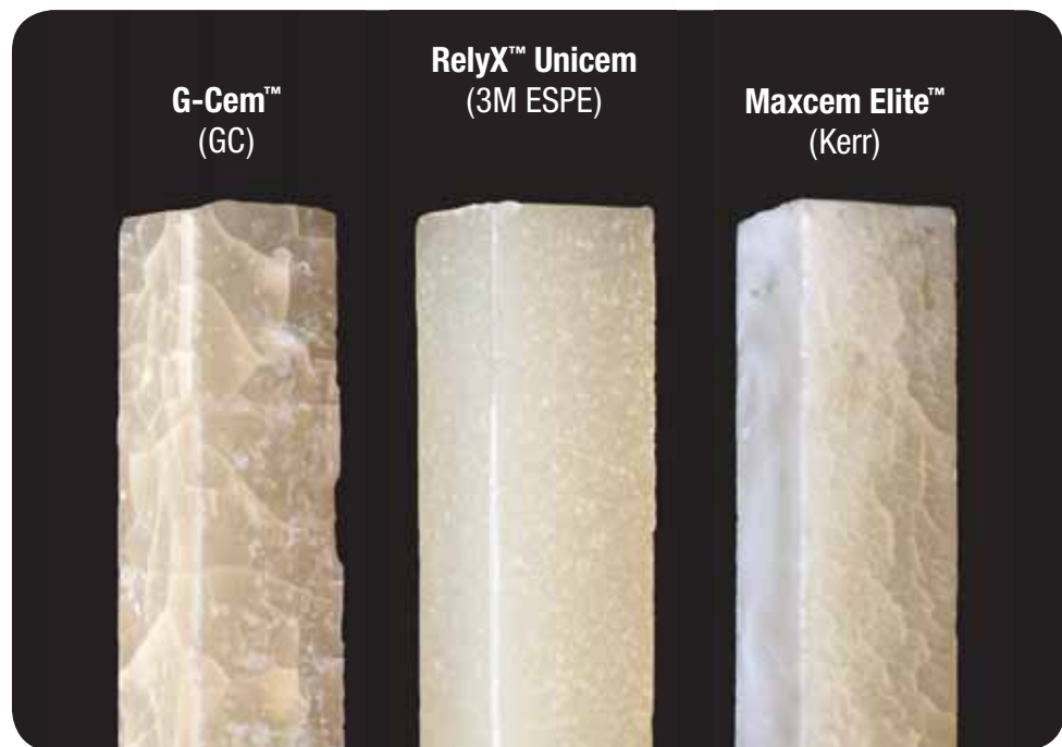
Results of thermocycling stress test on self-adhesive resin cements. Source: 3M ESPE internal data
