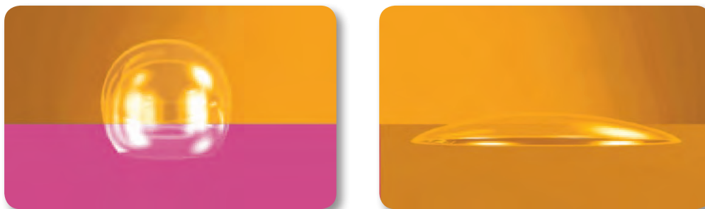
Fig. 5: Hydrophobic (left) versus hydrophilic behavior of a water droplet on impression material (schematic pictures).
