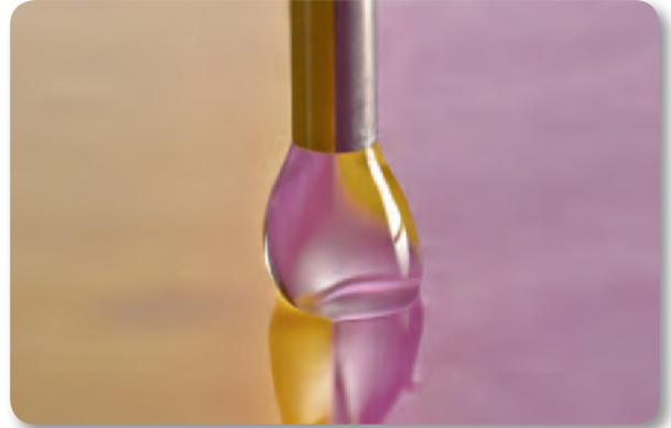
Fig. 11: ... to the interface of two unset light body VPS impression materials (40 sec. after start of mixing). All measurements were performed at room temperature (23°C/73.4°F).
