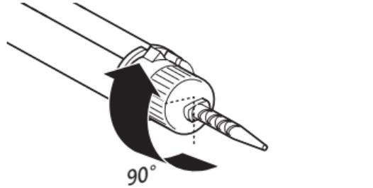
1. Before attaching the mixing tip, remove the cap [A] or used mixing tip after turning it 90° counterclockwise, and discard it.
