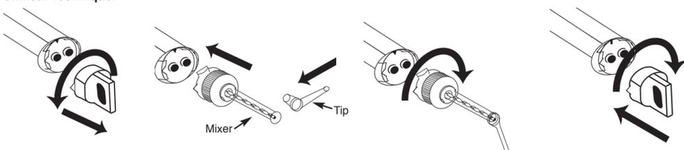
1. Remove the syringe cap, place the mixing stator on the syringe and place the delivery tip onto the mixing stator.
